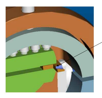
The bit cutting edge need to toward the Push Type Broach Bolt.
