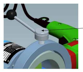
Step 1: Rotate the handle to the outside of collect. Use fingers to push it from inside untill it fall out.
