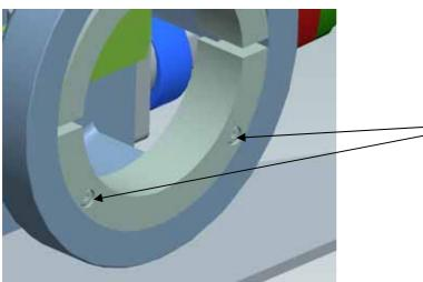
Step 2: Screw out two screw bolts with inner hexagonal wrench, then take out the lower mold of collect.
