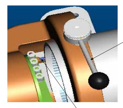
Rotate the handle to tighten the pipe
